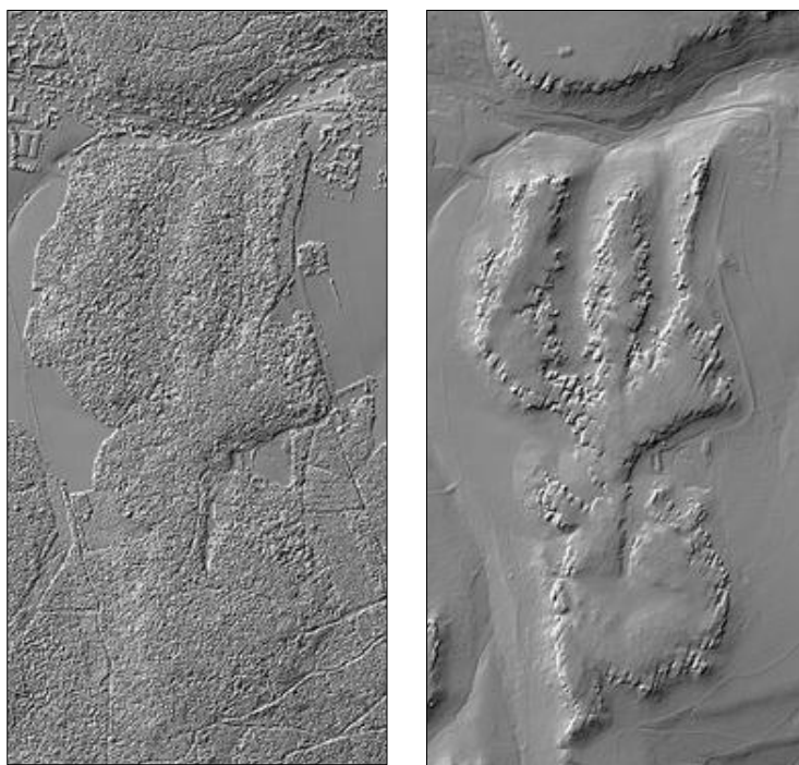
Fig. 2. Digital canopy surface model (left) and digital terrain model (right) of the forested landscape of the cliffs of the Nikolsdorfer Wände (Elbe Sandstone Mountains) © EU-INTEREG-III A – GENESIS, IPF-TUD).
